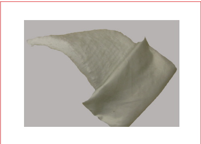
Fire Blanket To protect superwool from tearing. Treated with a non flammable vinyl acetate solution. Cloth will withstand 500°C but at 200°C weavelock will disperse. Available in rolls 1m x 50m
