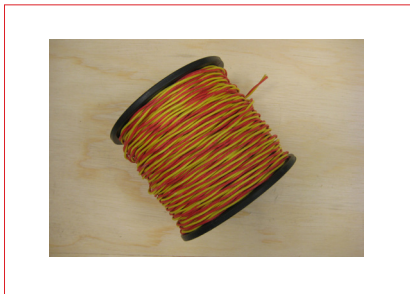
Thermocouple Wire Comes in 100m reels. Used for temperature measurement
