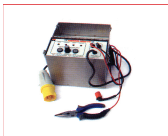
Thermocouple Attachment Unit
