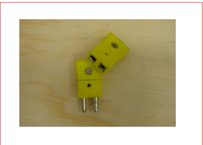
Thermocouple Plugs To connect thermocouple wire to extensions and Rapidheat machines
